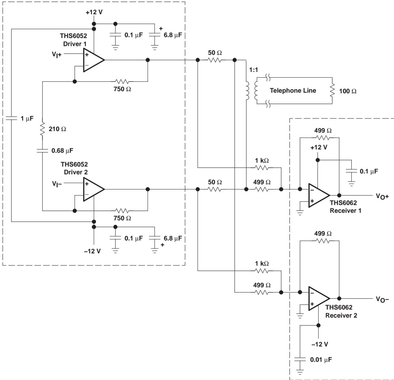
Figure 1. THS6052 ADSL Application With 1:1 Transformer Ratio
