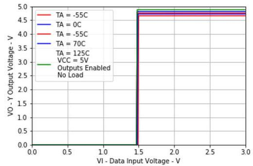
**Figure 5-3. Y Output Voltage vs Data Input Voltage**
