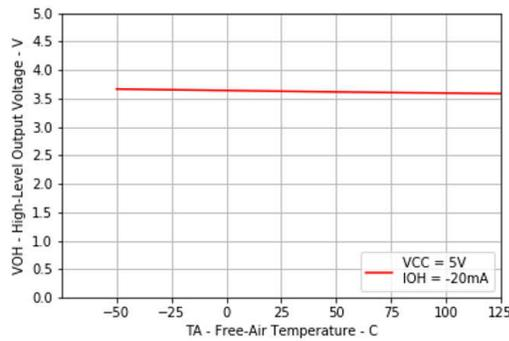
Figure 5-8. High-level Output Voltage vs Free-air Temperature
