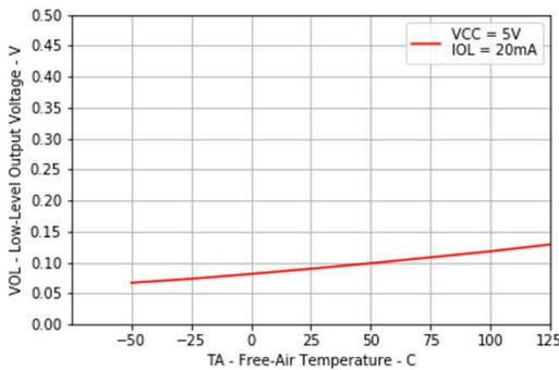
Figure 5-10. Low-level Output Voltage vs Free-air Temperature
