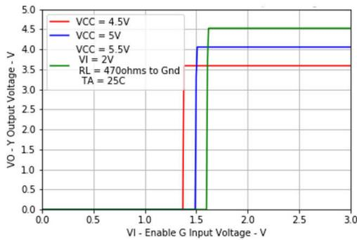
**Figure 5-2. Y Output Voltage vs Data Input Voltage**
