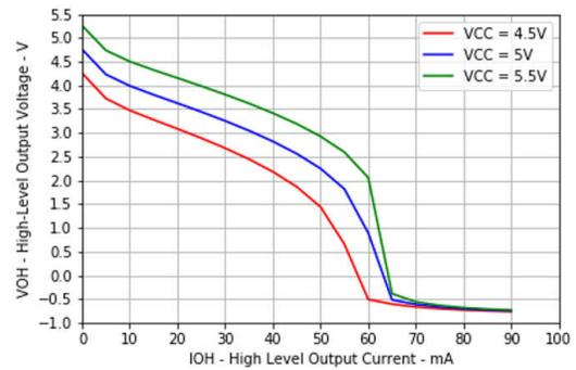
Figure 5-9. High-level Output Voltage vs High-level Output Current
