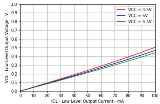
Figure 5-11. Low-level Output Voltage vs Low-level Output Current
