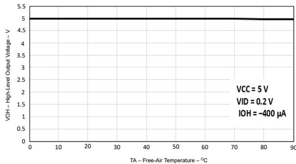
**Figure 5-3. High-level Output Voltage vs Free-air Temperature 5**
