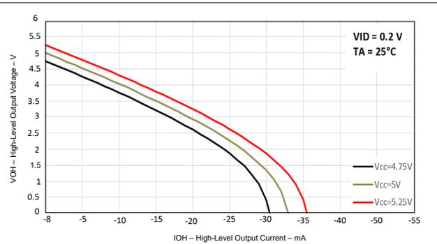
**Figure 5-2. High-level Output Voltage vs High-level Output Current**
