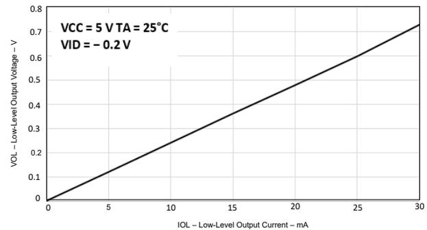
**Figure 5-4. Low-level Output Voltage vs Low-level Output Current**
