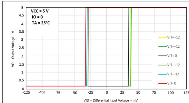
**Figure 5-1. Output Voltage vs Differential Input Voltage**
