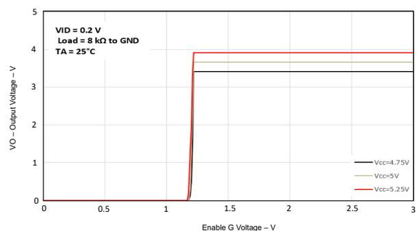
**Figure 5-6. Output Voltage vs Enable G Voltage**
