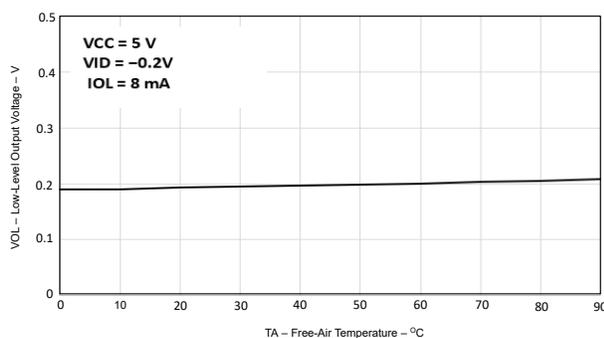
**Figure 5-5. Low-level Output Voltage vs Free-air Temperature**
