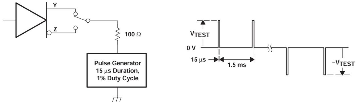
Figure 6-8. Test Circuit and Waveform, Transient Over-Voltage
