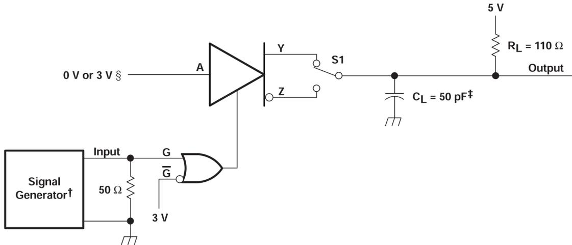
† PRR = 1 MHz, 50% duty cycle,  $t_r < 6$  ns,  $t_f < 6$  ns,  $Z_O = 50 \Omega$
