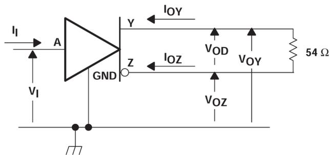
Figure 6-1. Test Circuit,  $V_{OD}$  Without Common-Mode Loading
