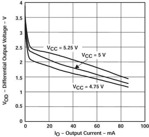
Figure 5-1. Differential Output Voltage vs Output Current
