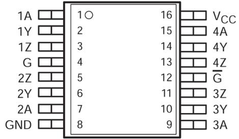
**Figure 4-2. 16-DW Package (Top View)**
