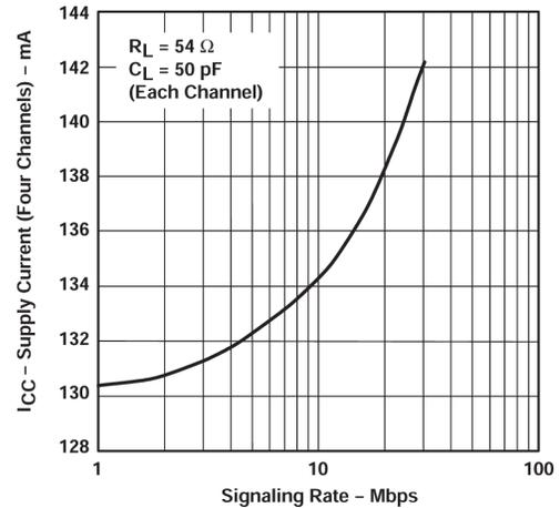
Figure 5-4. Supply Current (Four Channels) vs Signaling Rate
