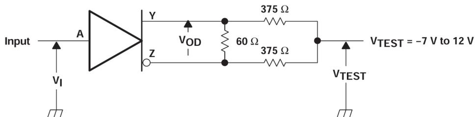
Figure 6-2. Test Circuit,  $V_{OD}$  With Common-Mode Loading
