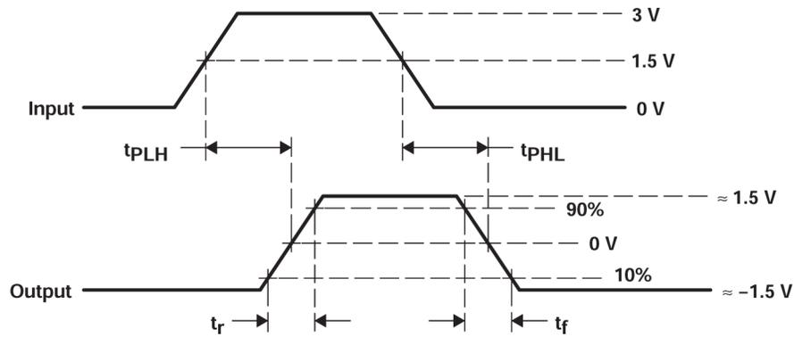
**Figure 6-4. Output Switching Test Circuit and Waveforms**
