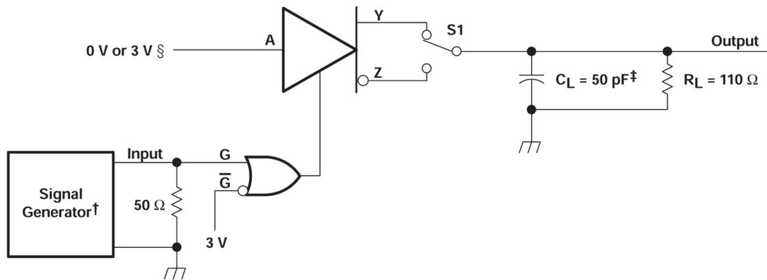
† PRR = 1 MHz, 50% duty cycle,  $t_r < 6$  ns,  $t_f < 6$  ns,  $Z_O = 50 \Omega$
