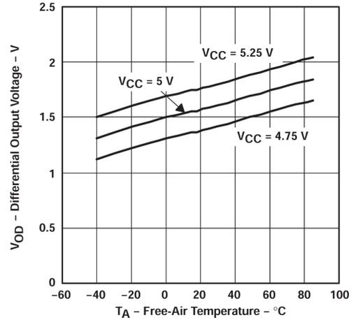
Figure 5-2. Differential Output Voltage vs Free-air Temperature
