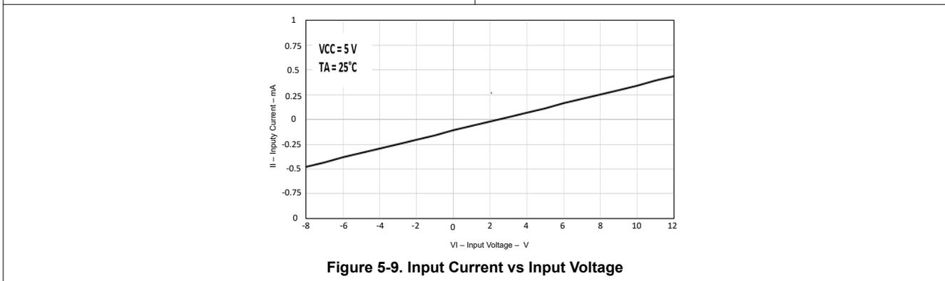
Figure 5-9. Input Current vs Input Voltage
