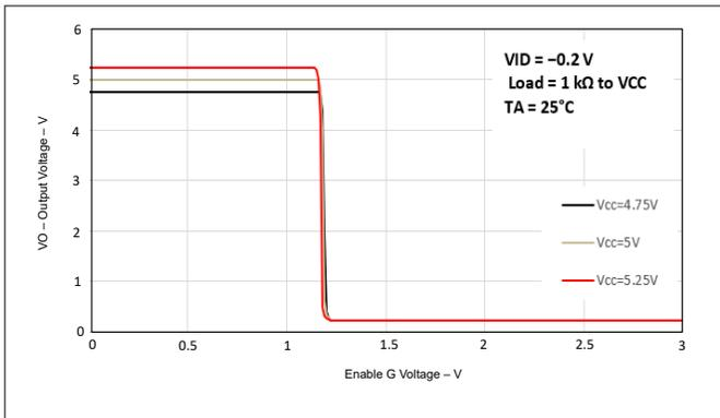
Figure 5-7. Output Voltage vs Enable G Voltage
