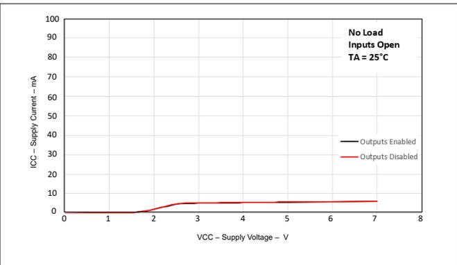
Figure 5-8. Supply Current (All Receivers) vs Supply Voltage
