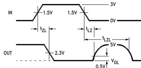
**Note 8:**The input pulse is supplied by a generator having the following characteristics:  $f = 1.0 \text{ MHz}$ , duty cycle = 50%,  $t_r \leq 5.0 \text{ ns}$ ,  $t_f \leq 5.0 \text{ ns}$ ,  $Z_O = 50\Omega$ .
