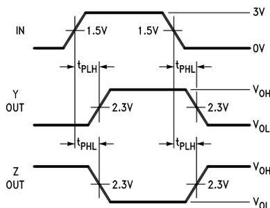
**Note 8:** The input pulse is supplied by a generator having the following characteristics:  $f = 1.0 \text{ MHz}$ , duty cycle = 50%,  $t_r \leq 5.0 \text{ ns}$ ,  $t_f \leq 5.0 \text{ ns}$ ,  $Z_O = 50 \Omega$ .
