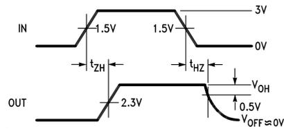
**Note 8:**The input pulse is supplied by a generator having the following characteristics:  $f = 1.0 \text{ MHz}$ , duty cycle = 50%,  $t_r \leq 5.0 \text{ ns}$ ,  $t_f \leq 5.0 \text{ ns}$ ,  $Z_O = 50\Omega$ .
