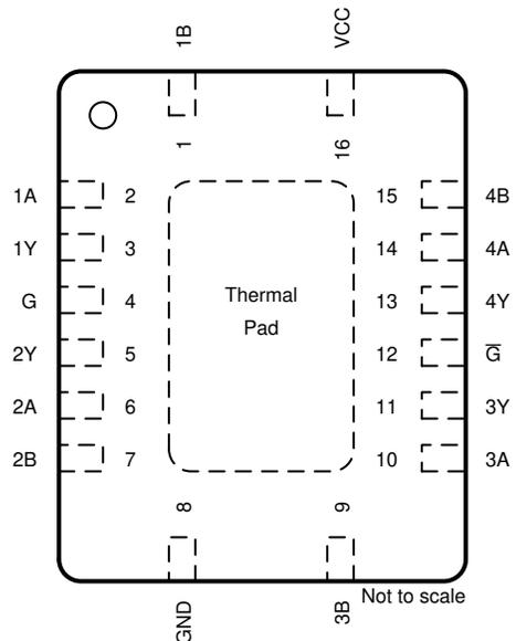
**Figure 5-2. RGY Package 16-Pin VQFN (Top View)**
