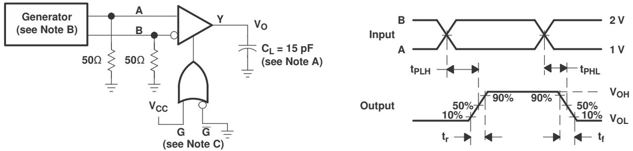
A.  $C_L$  includes probe and jig capacitance.
