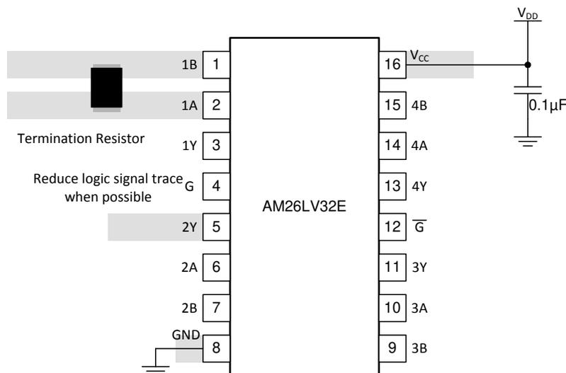
Figure 11-1. Trace Layout on PCB and Recommendations
