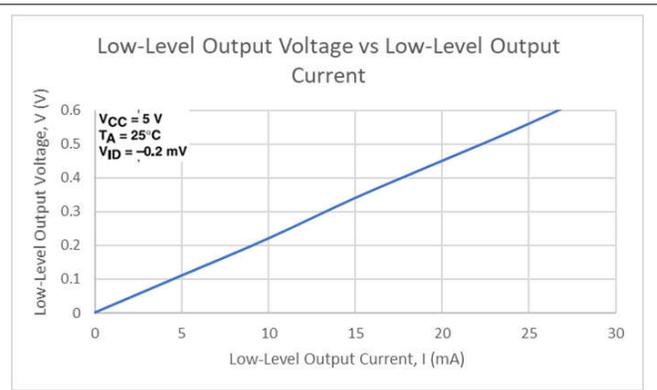
**Figure 6-2. Low-Level Output Voltage vs Low-Level Output Current**
