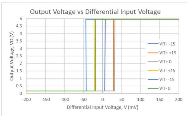
**Figure 6-9. AM26LS33A Output Voltage vs Differential Input Voltage**
