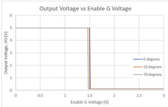
**Figure 6-7. Output Voltage vs Enable G Voltage**
