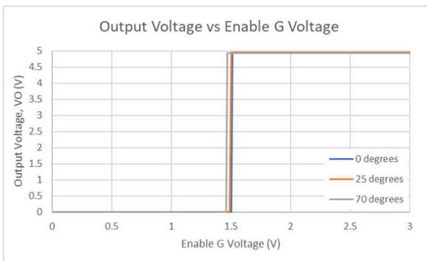
**Figure 6-5. Output Voltage vs Enable G Voltage**
