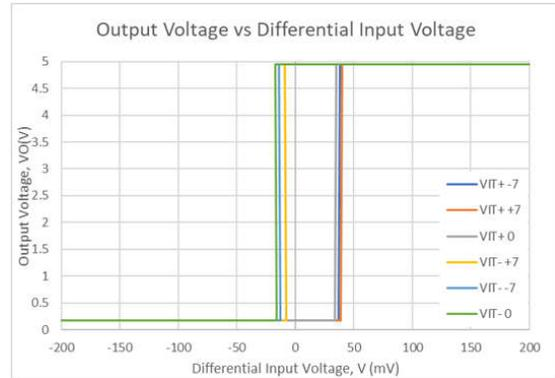
**Figure 6-8. AM26LS32A Output Voltage vs Differential Input Voltage**
