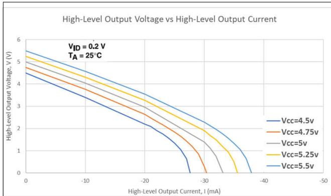
**Figure 6-1. High-Level Output Voltage vs High-Level Output Current**
