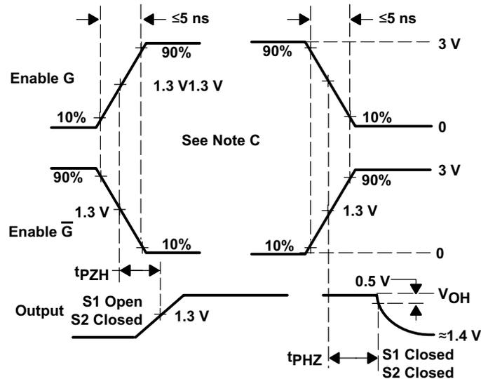
Figure 7-3. Voltage Waveforms For  $t_{PHZ}$ ,  $t_{PZH}$
