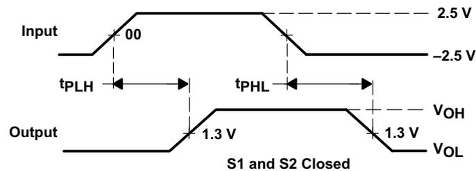
Figure 7-2. Voltage Waveforms For  $t_{PLH}$ ,  $t_{PHL}$
