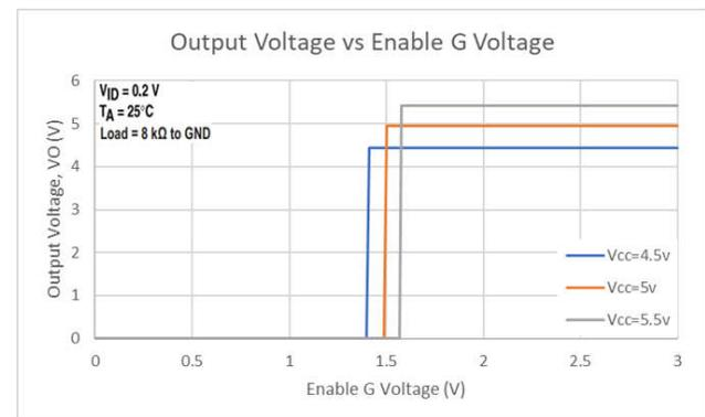
**Figure 6-4. Output Voltage vs Enable G Voltage**
