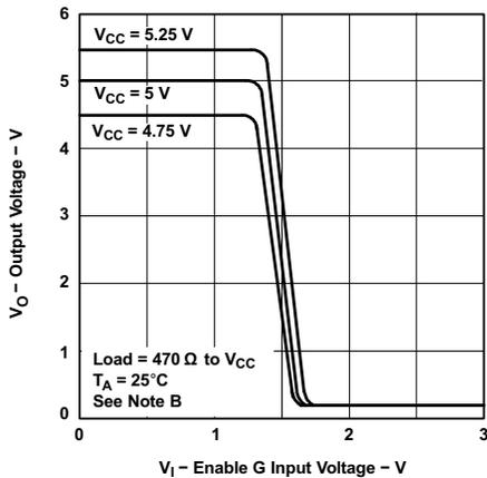
B. The A input is connected to ground during testing of the Y outputs and to  $V_{CC}$  during testing of the Z outputs.
