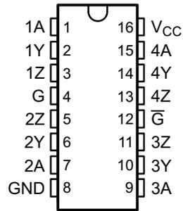
**Figure 4-1. D (SOIC), DB (SSOP), N (PDIP) , NS (SO), J (CDIP), or W (CFP) Packages
