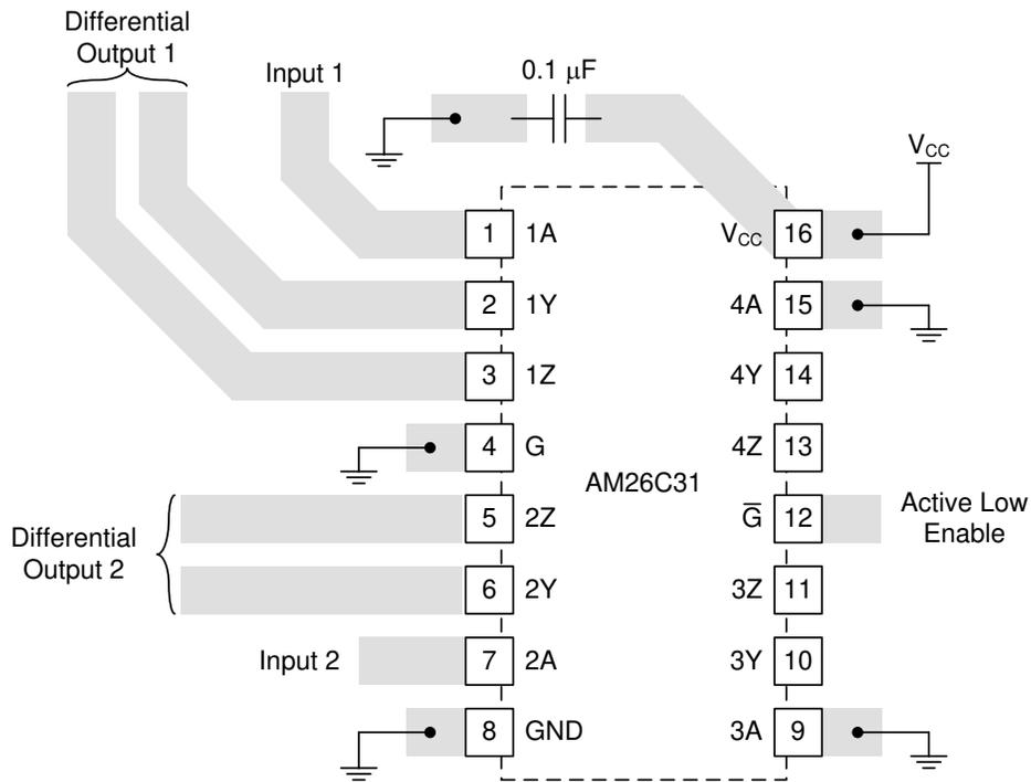
**Figure 8-3. Trace Layout on PCB and Recommendations**
