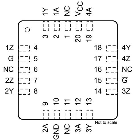
Figure 4-2. FK (LCCC) Package, 20-Pin (Top View)
