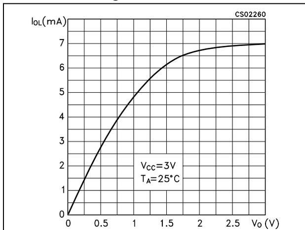
**Figure 6. Output current vs. output high voltage**
