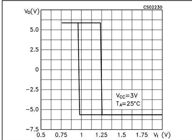
**Figure 4. Driver voltage transfer characteristics for receiver inputs**
