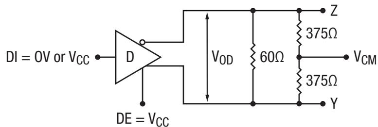
Figure 4. Differential Driver Output Voltage Over Common Mode
