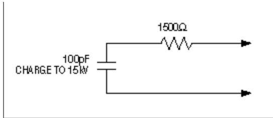
Figure 2. When discharged, this circuit (the Human Body Model) produces a very fast rise time with current peaks of 15kV/1.5kΩ—over 10A!
