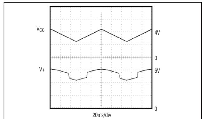
Figure 1. V+ Switchover for Changing V<sub>CC</sub>
