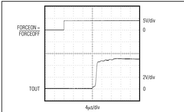
Figure 7. Transmitter Outputs Exiting Shutdown or Powering Up
