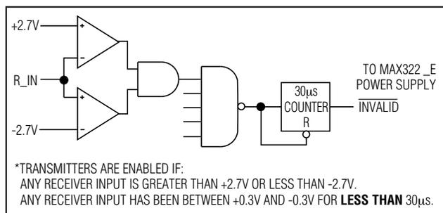
Figure 2b. MAX322\_E with Transmitters Enabled Using AutoShutdown
