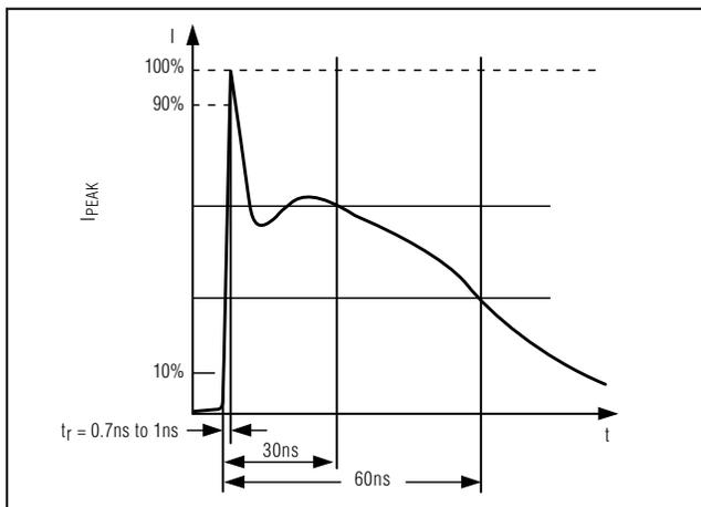
Figure 6b. IEC 1000-4-2 ESD Generator Current Waveform
