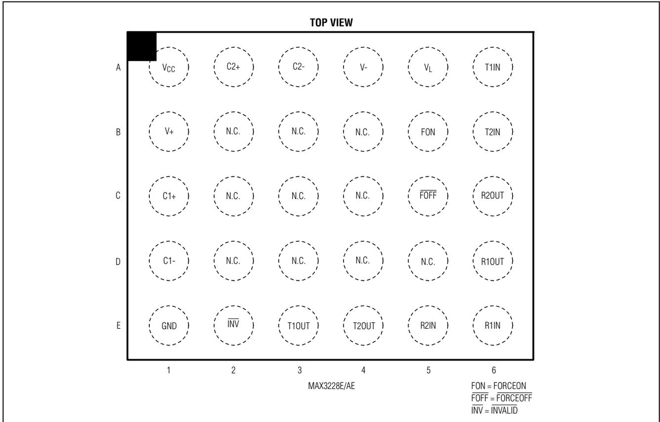
**±15kV ESD-Protected +2.5V to +5.5V RS-232 Transceivers in UCSP and WLP**
