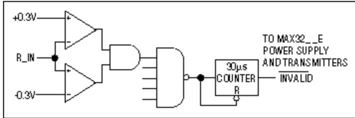
Figure 3. Autoshtutdown is entered if all receivers' inputs are between +/-0.3V for at least 30µS.
