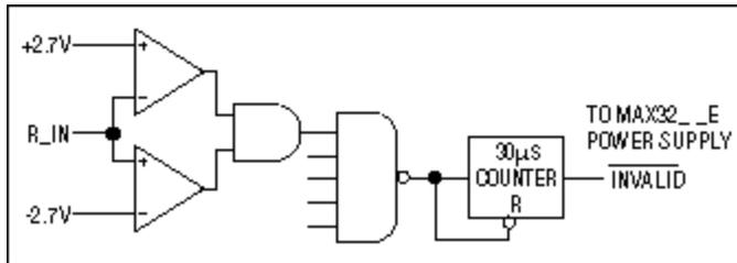
Figure 4. Autoshtutdown is exited if any receiver exceeds +/-2.7V.
