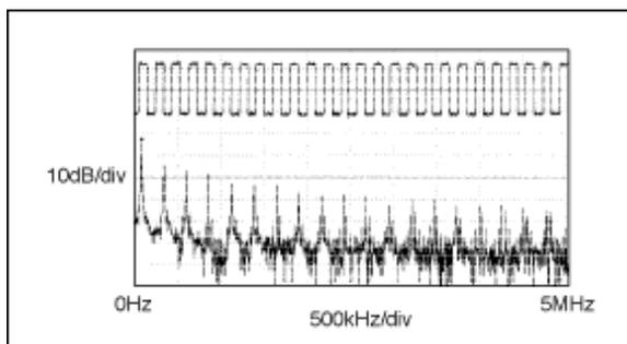
Figure 2. The driver output waveform and FFT plot of the MAX3485E/MAX3490E/MAX3491E transmitting a  $125\text{kHz}$  signal.
