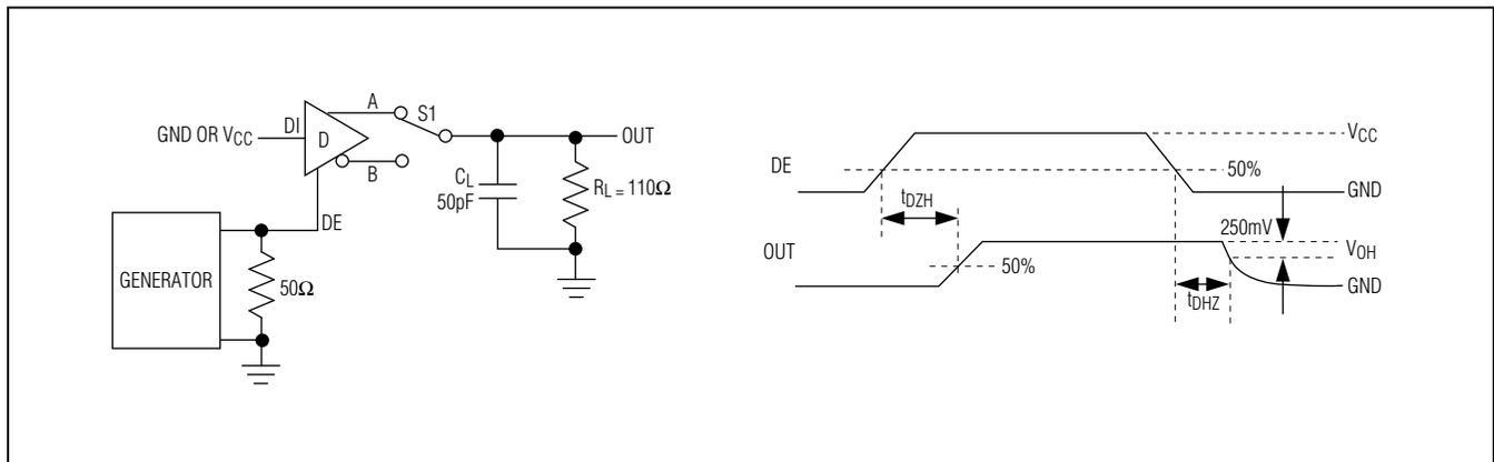
Figure 4. Driver Enable and Disable Times ( $t_{DZH}$ ,  $t_{DZL}$ )
