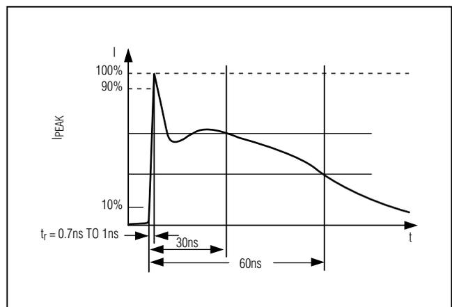
Figure 13. IEC 61000-4-2 ESD Generator Current Waveform
