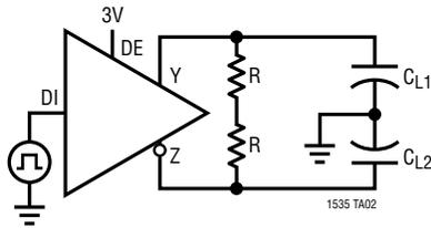
Figure 19. Fail-Safe Logic "0"
