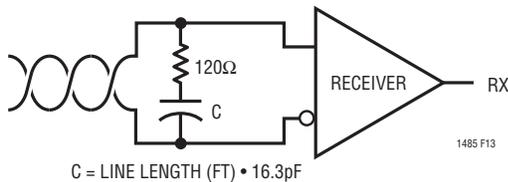
Figure 13. AC-Coupled Termination
