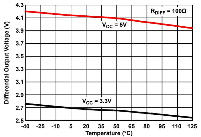
Figure 9. Driver Differential Output Voltage vs Temperature
