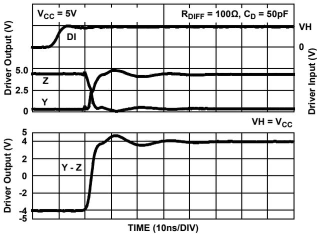
Figure 18. Driver Waveforms, Low to High
