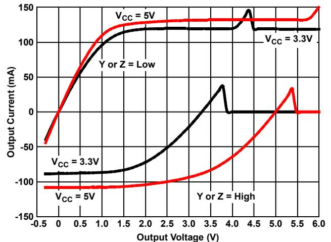
Figure 13. Driver Output Current vs Short-Circuit Voltage
