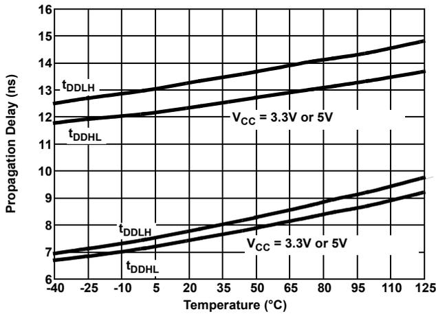
Figure 14. Driver Differential Propagation Delay vs Temperature
