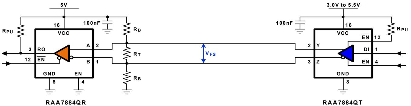
Figure 3. Network Using Group Enables
