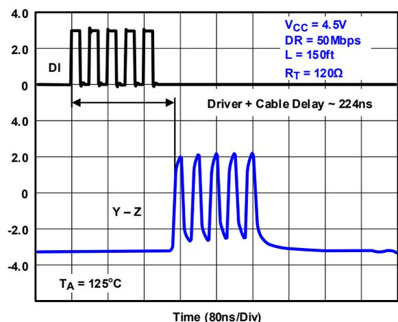
Figure 2. Data Rate Performance at 4.5V
