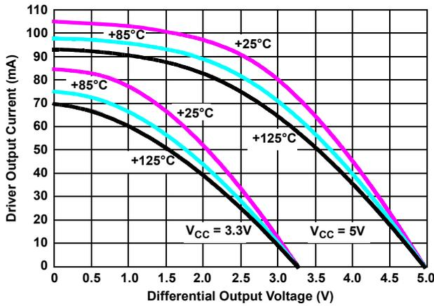
Figure 8. Driver Output Current Vs Differential Output Voltage
