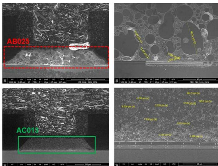
Figure 1. SEM images of the dispensing materials AB025 (current) and AC013 (new). Main difference is the sizes of the filler that could cause mechanical damage when product is subjected to high temperature solder reflow.
