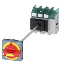
SENTRON, Molded case switch 3LD5 UL, Emergency switching-off, 4-pole, certified according to UL489 UL60947-4-1 and IEC60947-3, UL: 60A, SCCR 50kA at 480VAC, Operating power at 480VAC 3-phase: 40hp, IEC: 63A, Operating power at AC-23A at 400V: 30kW, floor mounting with door coupling rotary operating mechanism, defeatable, emergency switching-off, 4-hole mounting of the handle, without tolerance compensation, incl. terminal covers for the infeed side
