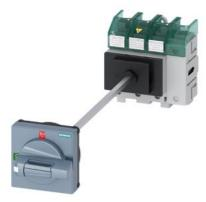
SENTRON, Molded case switch 3LD5 UL, Main switch, 4-pole, certified according to UL489 UL60947-4-1 and IEC60947-3, UL: 60A, SCCR 50kA at 480VAC, Operating power at 480VAC 3-phase: 40hp, IEC: 63A, Operating power at AC-23A at 400V: 30kW, floor mounting with door coupling rotary operating mechanism, defeatable, Standard, 4-hole mounting of the handle, without tolerance compensation, incl. terminal covers for the infeed side
