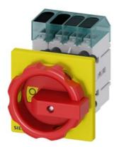
Load disconnector 3LD3, Iu 63 A Main switch 3-pole + N Rated operating capacity at AC-23 A at 400V 22.0 kW Front plate mounting Basic switch with Central hole mounting 22.5mm Toggle drive red / yellow 66x66 mm
