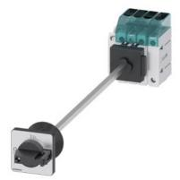
Load disconnector 3LD3, Iu 63 A Main switch 3-pole + N Rated operating capacity at AC-23 A at 400V 22.0 kW floor mounting Basic switch with door coupling Central hole mounting 22.5mm Toggle drive black 48x48 mm with auxiliary switch 1OE + 1S
