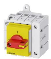
Load disconnector 3LD3, Iu 63 A Main switch 3-pole + N Rated operating capacity at AC-23 A at 400V 22.0 kW Installation in distribution boards, Basic switch with selector knob red / yellow with auxiliary switch 10E + 1S
