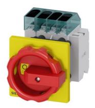
Load disconnector 3LD3, Iu 40 A Main switch 3-pole + N Rated operating capacity at AC-23 A at 400 V 18.5 kW Front plate mounting Basic switch with Central hole mounting 22.5mm Toggle drive red / yellow 66x66 mm with auxiliary switch 10E + 1S
