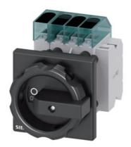
Load disconnector 3LD3, lu 40 A Main switch 3-pole + N Rated operating capacity at AC-23 A at 400 V 18.5 kW Front plate mounting Basic switch with Central hole mounting 22.5mm Toggle drive black 66x66 mm with auxiliary switch 1OE + 1S
