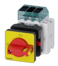
Load disconnector 3LD3, lu 40 A Main switch 3-pole Rated operating capacity at AC-23 A at 400 V 18.5 kW Front plate mounting Basic switch with Central hole mounting 22.5mm Toggle drive red / yellow 48x48 mm with auxiliary switch 1OE + 1S
