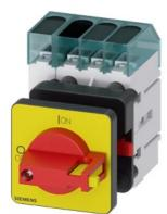
Load disconnector 3LD3, Iu 40 A Main switch 3-pole + N Rated operating capacity at AC-23 A at 400 V 18.5 kW Front plate mounting Basic switch with Central hole mounting 22.5mm Toggle drive red / yellow 48x48 mm
