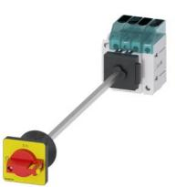
Load disconnector 3LD3, Iu 40 A Main switch 3-pole + N Rated operating capacity at AC-23 A at 400 V 18.5 kW floor mounting Basic switch with door coupling Central hole mounting 22.5mm Toggle drive red / yellow 48x48 mm with auxiliary switch 10E + 1S
