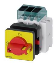
Load disconnector 3LD3, lu 32 A Main switch 3-pole Rated operating capacity for AC-23 A at 400V 11.5kW Front plate mounting Basic switch with Central hole mounting 22.5mm Toggle drive red / yellow 48x48 mm with auxiliary switch 1OE + 1S
