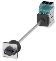
Load disconnector 3LD3, Iu 32 A Main switch 3-pole Rated operating capacity for AC-23 A at 400V 11.5kW floor mounting Basic switch with door coupling Central hole mounting 22.5mm Toggle drive black 48x48 mm
