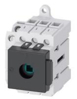
Load disconnector 3LD3, Iu 32 A Main switch 3-pole Rated operating capacity for AC-23 A at 400V 11.5kW Installation in distribution boards, Basic switch without Knob-operated mechanism with auxiliary switch 10E + 1S
