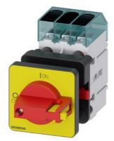
Load disconnector 3LD3, lu 25 A Main switch 3-pole Rated operating capacity at AC-23 A at 400V 9.0kW Front plate mounting Basic switch with Central hole mounting 22.5mm Toggle drive red / yellow 48x48 mm
