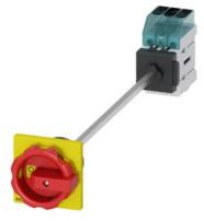
Load disconnector 3LD3, lu 25 A Main switch 3-pole Rated operating capacity at AC-23 A at 400V 9.0kW floor mounting Basic switch with door coupling Central hole mounting 22.5mm Rotary actuator red / yellow 66 x 66 mm
