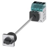
Load disconnector 3LD3, lu 25 A Main switch 3-pole + N Rated operating capacity at AC-23 A at 400V 9.0kW floor mounting Basic switch with door coupling Central hole mounting 22.5mm Toggle drive black 48x48 mm
