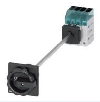
Load disconnector 3LD3, lu 16 A Main switch 3-pole + N Rated operating capacity at AC-23 A at 400V 7.5kW floor mounting Basic switch with door coupling Central hole mounting 22.5mm Rotating drive black 66 x 66 mm
