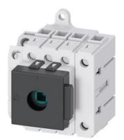
Load disconnector 3LD3, lu 16 A Main switch 3-pole + N Rated operating capacity at AC-23 A at 400V 7.5kW Installation in distribution boards, Basic switch without Knob-operated mechanism with auxiliary switch 1OE + 1S
