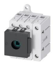
Load disconnector 3LD3, lu 16 A Main switch 3-pole + N Rated operating capacity at AC-23 A at 400V 7.5kW Installation in distribution boards, Basic switch without Knob-operated mechanism
