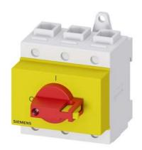
SENTRON, Switch disconnector 3LD, emergency switching-off switch, 3- pole, lu: 125 A, operating power / at AC-23 A 400 V: 45 kW, installation in distribution boards, knob-operated mechanism, Red / yellow, handle direct at the switch
