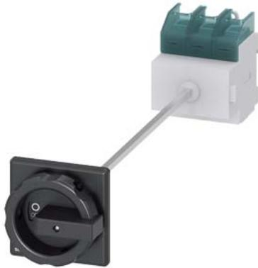
SENTRON, Switch disconnecter 3LD, main switch, 3-pole, Iu: 100 A, Operating power / at AC-23 A at 400 V: 37 kW, floor mounting with door coupling, rotary operating mechanism, black, 4-hole mounting of the handle
