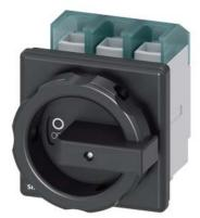
SENTRON, Switch disconnector 3LD, main switch, 3-pole, lu: 100 A, Operating power / at AC-23 A at 400 V: 37 kW, front-mounted, rotary operating mechanism, black, 4-hole mounting of the handle
