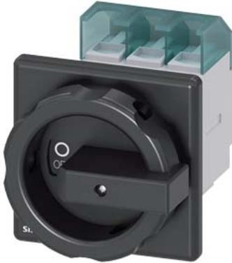
SETRON, Switch disconnecter 3LD, main switch, 3-pole, Iu: 63 A, Operating power / at AC-23 A at 400 V: 22 kW, front-mounted, rotary operating mechanism, black, central mounting 22.5 mm of the handle
