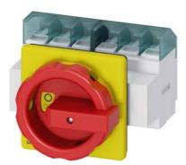
SENTRON, Switch disconnector 3LD, emergency switching-off switch, 6- pole, lu: 63 A, operating power / at AC-23 A 400 V: 22 kW, front-mounted, rotary operating mechanism, Red / yellow, 4-hole mounting of the handle
