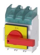
SENTRON, Switch disconnector 3LD, emergency switching-off switch, 3- pole, Iu=250 A, operating power / at AC-23 A 400 V: 132 kW, installation in distribution boards, knob-operated mechanism, Red / yellow, handle direct at the switch
