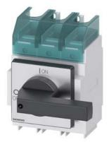
SENTRON, Switch disconnector 3LD, main switch, 3-pole, lu=250 A, Operating power / at AC-23 A at 400 V: 132 kW, installation in distribution boards, knob-operated mechanism, black, handle direct at the switch
