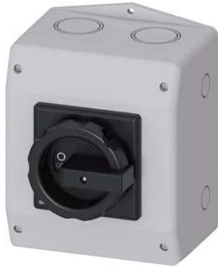
SETRON, Switch disconnecter 3LD, main switch, 6-pole, Iu: 32 A, Operating power / at AC-23 A at 400 V: 11.5 kW, molded-plastic encapsulation for metric screw connection, 1 NC, 1 NO, rotary operating mechanism, black
