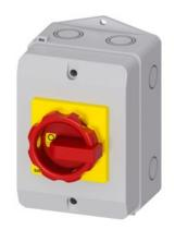
SENTRON, Switch disconnector 3LD, emergency switching-off switch, 3- pole, lu: 32 A, operating power / at AC-23 A 400 V: 11.5 kW, molded-plastic encapsulation for inch cable gland, 2 NO, rotary operating mechanism, red/yellow
