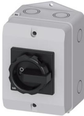
SETRON, Switch disconnecter 3LD, main switch, 3-pole, Iu: 32 A, Operating power / at AC-23 A at 400 V: 11.5 kW, molded-plastic encapsulation for inch cable gland, rotary operating mechanism, black
